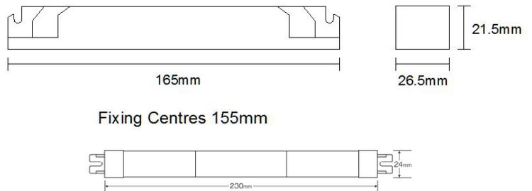
The HLP/1S is supplied as a maintained/non-maintained emergency driver for integral mounting within a luminaire.
