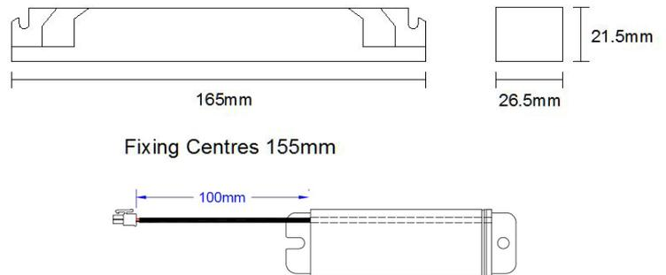
The HLP/1 is supplied as a maintained/non-maintained emergency driver for integral mounting within a luminaire.
